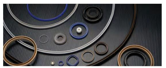
Exceptionally durable, our specially designed PTFE-based sealing jacket, Metaplast II spring, and a patented metallic C-shaped spring conform the Metaplast II spring seal. Available in eight standard cross sections for O-ring and custom groove designs in diameters from 1/8" to 60", and 3.25mm to 1500mm.
