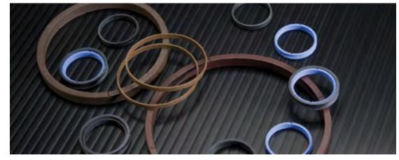
Elastomer-energized PTFE seals have many years of successful operation in hydraulic and pneumatic systems. The polymer-based dynamic sealing element is used with an elastomer acting as a static energizer. Available in custom designs and 13,000 standard inch and metric sizes conforming to industrial and military specifications.
