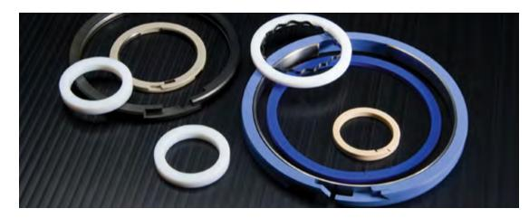
Patented one-piece piston ring with unique step cut joint. While the Tetraflex Piston rings employ either a metallic wave spring or a flat-ribbon energizer, the Tetraflex II Piston ring makes use of an enclosed expander clip which easily facilitates handling and installation. We can also make individual designs for all military and industrial hydraulic systems.
