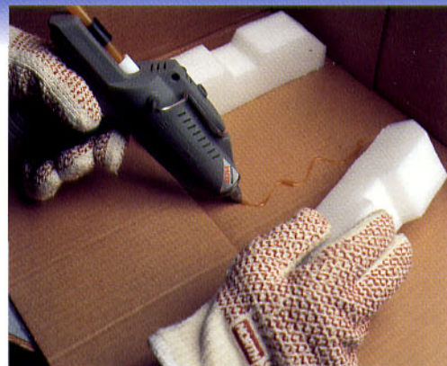
New Bostik 660G gun and 2109 glue sticks speed assembly of foam to corrugated for packaging fabrication.
