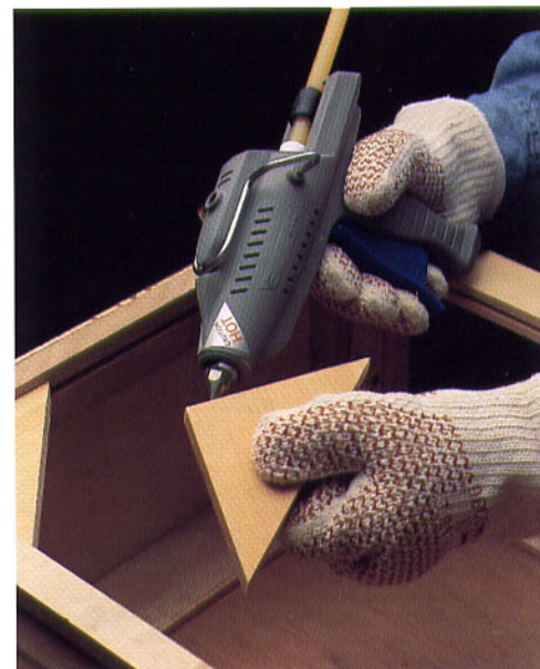
Bostik's 660G gun and 0120 glue sticks create long-lasting bonds in wood drawer assembly.
