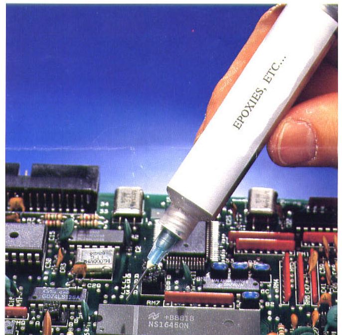
Bonding components with electrically conductive epoxy.
