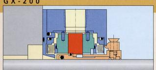
**Maximum Operating Limits** 200 psi / 13.8 bar Pressure: 1000 / 69 500°F / 260°C Temperature: 800 / 427 500 to 7000 fpm / 2.5 to 35 m/s Speed: 0/0 10000 / 51 1.000" to 3.000" / 25 mm to 75 mm Sizes: 0/0 12.000 / 305
