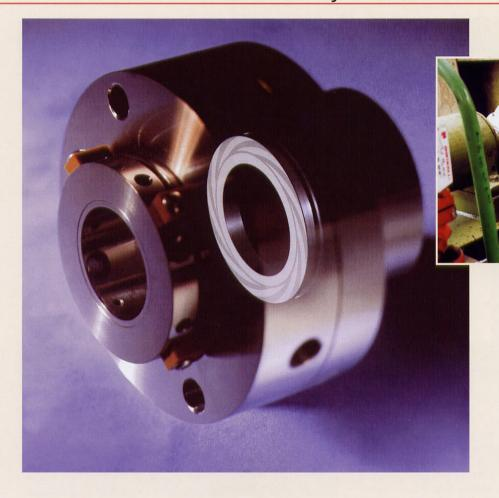
as seal technology and gas seal operation depends on aerostatic and aerodynamic forces, Careful design keeps the two faces separated by a gas film of 40-80 µin /1-2 µm. Aerodynamic forces are created by the presence of a 'pattern' on one of the faces. Flowserve uses:
