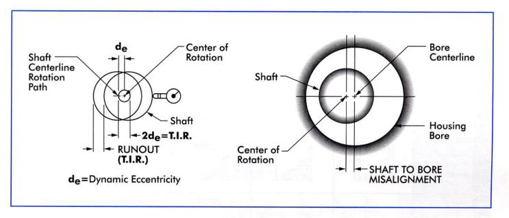
Eccentricity is determined by measuring the shaft runout, TIR, and the shaft-to-bore misalignment. Combine the two results for the total eccentricity the seal lip must follow to
