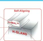
Self Aligning No retainer rings needed which simplifies assembly H-Seals work 100% of the time. Guaranteed! and saves money.
